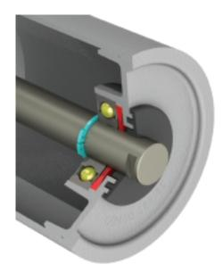
Link-Belt® E2000 rolls are designed for the rugged, maximum capacity and continuous handling requirements of heavy, coarse and abrasive materials such as coal, iron ore, copper, large stone and overburden. Featuring an exceptionally robust seal design and 40 mm ball bearings, E2000 rolls are available for belt widths from 36 to 96 inches, and 20°, 35° and 45°troughed belt idlers, flat return and v-return idlers in 6" and 7" diameters.
