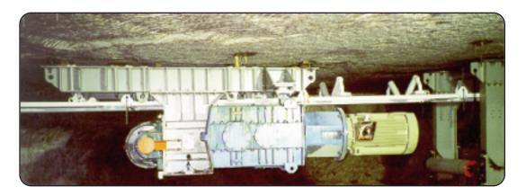
Roof-Mount 2-Pulley Alignment-Free Drive
