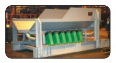
Syntron Material Handling offers Link-Belt intermediate loading sections for all transition angles, with associated chute and skirt arrangements.
