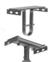
No. 270 ball bearing hangers have self-aligning ball bearings. The frame is a box-member top-bar with a pipe stem support for the bearing. The bearing is factory adjusted for the proper length from the top-bar and locked with a sealant and a lock nut. The frame is designed for mounting inside the trough and slotted mounting holes parallel to the conveyor permit adjustment and alignment.
