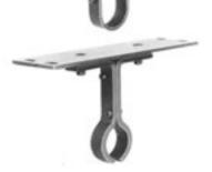
No. 220 hangers are similar in construction to No. 226 hangers, except they are mounted on top of the trough flanges. Mounting holes are slotted parallel with the conveyor to provide adjustment and alignment. These hangers are normally furnished with hard iron, babbitted, bronze, oil impregnated wood or molded fabric bearings, but can also be furnished with special bearings.
