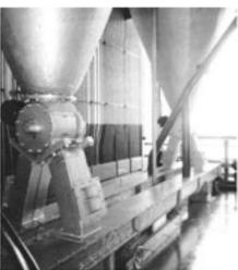
**Bottom:** Helicoid screw conveyors are essential components in this flour collecting system located in a large bakery.
