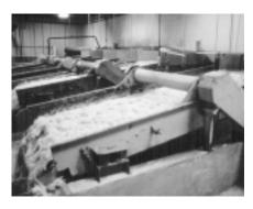
Four Link-Belt<sup>®</sup> Model NRM liquid Vibrating screens dewatering feathers and offal in a chicken processing plant.
