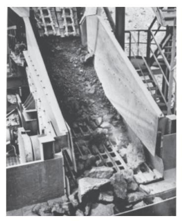
Link-Belt<sup>®</sup> Model BA heavy duty vibrating screen scalping iron ore. 4" and under passes through screen to a feeder while oversize travels over screen to crusher.
