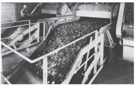
Two Link-Belt® Model SG2616 straightline vibrating screens washing and sizing coal.
