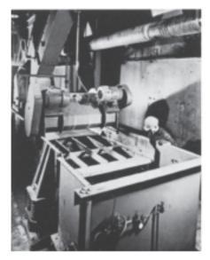
Link-Belt® Model SS2416 two-deck vibrating screen dewatering coal refuge.
