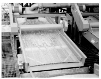
Single-deck NRM dewatering screen at a fish hatchery.
