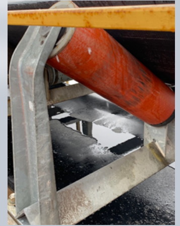
Composite roll with galvanized frame, 3 years over salty water!
