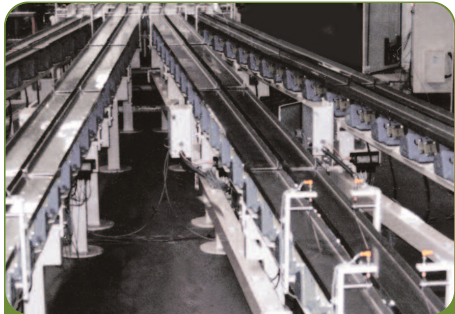
Custom designed sandwiching processes rely on Syntron drives to ensure consistent, controlled delivery and smooth, gentle cookie, wafer or cracker handling.
